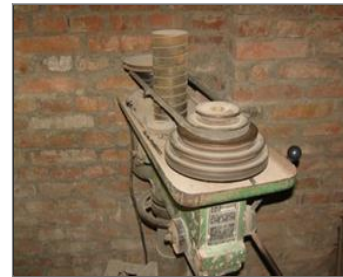
Photo of the inside of the main production hall NC-no belt guard for drilling machine.JPG
